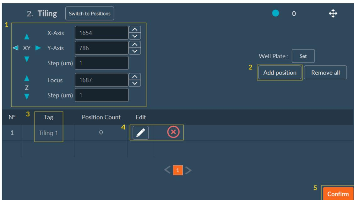
1. Move the stage and the focus to the desired position.
