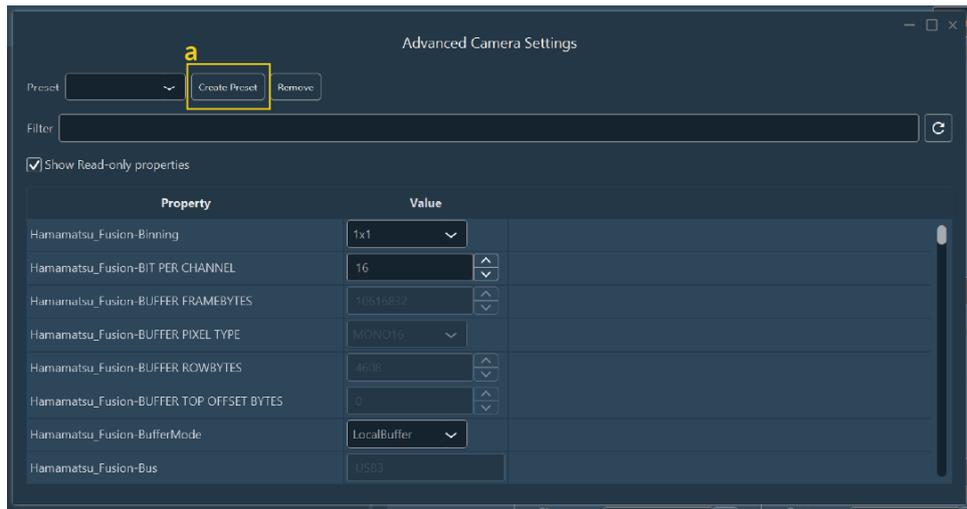
b. Select the parameters which will be saved in the camera preset by checking boxes. You can filter the parameters by writing in the search bar.
