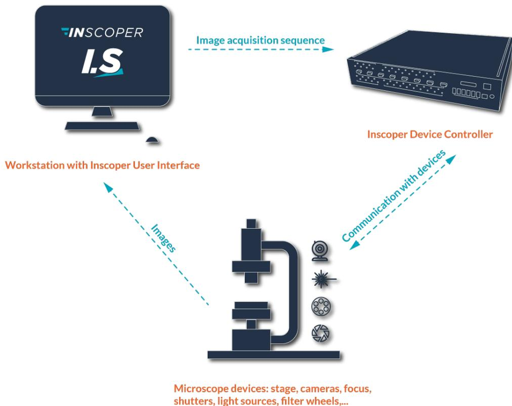
This separation means that the Inscoper I.S. is free from hardware constraints. Therefore, regardless of the type of microscope, the Interface remains simple, easy to use and focused on user requirements rather than hardware issues.
