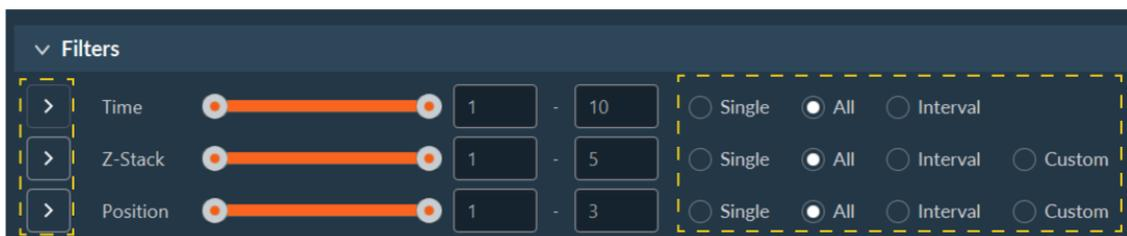
The Inscoper I.S. offers various tools to facilitate navigation between images, such as filters for example. In the **Filters** section, you can select a single image, a group or all images. The **Play** button next to the dimension name allows you to replay the selected sequence.
