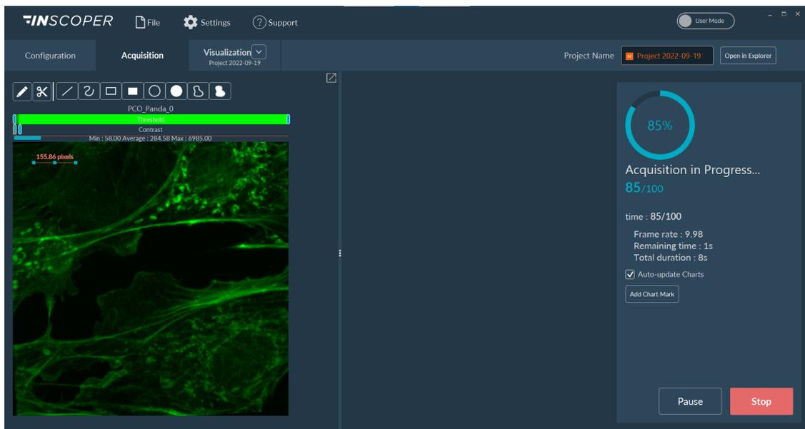
You can monitor the acquisition sequence while it is running. The left part of the window shows the current images of the sequence. The middle part is reserved for graphics if needed (not here). And in the right part of the window, you can follow the progress of the acquisition, pause or stop the sequence.
