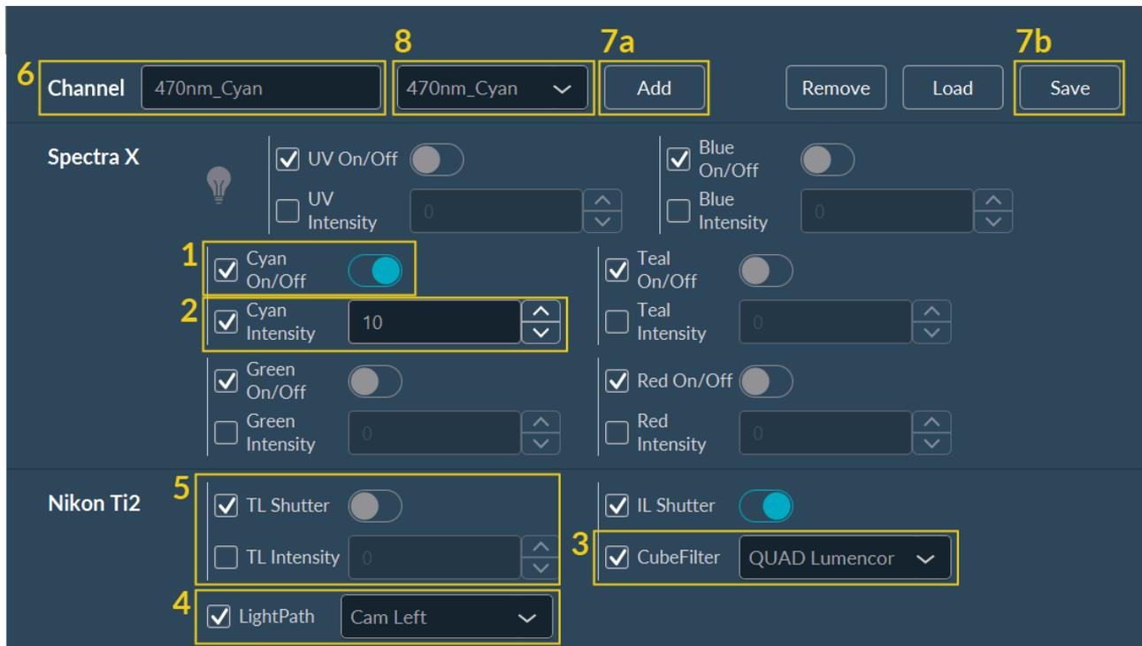
The expert users (if this option is activated) have access to all optical motorized elements of the microscope, like wheel filter, dichroic cube and light source. To manually create a fluorescent channel, you should follow the steps below:
