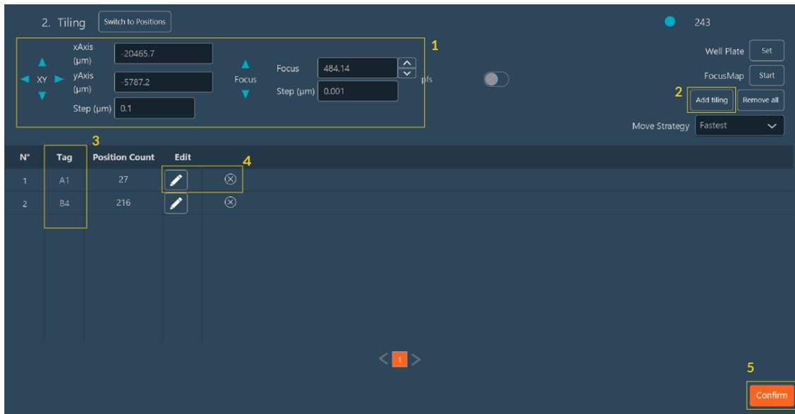
1. Move the stage and adjust the focus to the desired position.
