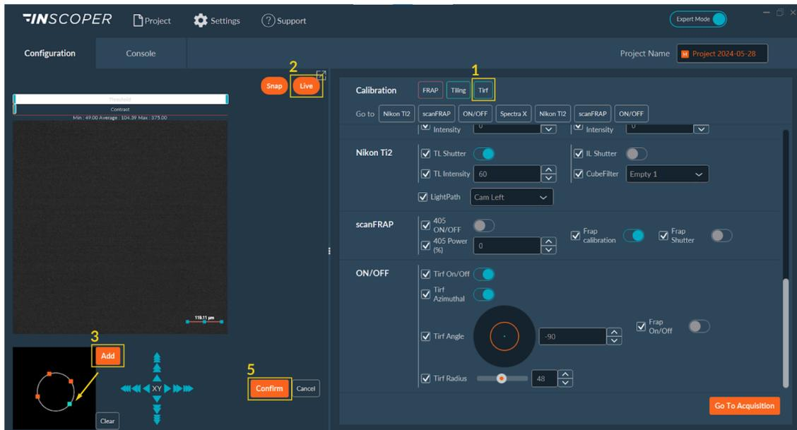
1. Click on **Tirf** button in the Calibration section.
