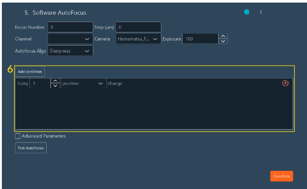
7. Check **Advanced Parameters** to set up the device to do the autofocus (for example, the piezo or the focus of the microscope) and if you need to apply offset to another device.
