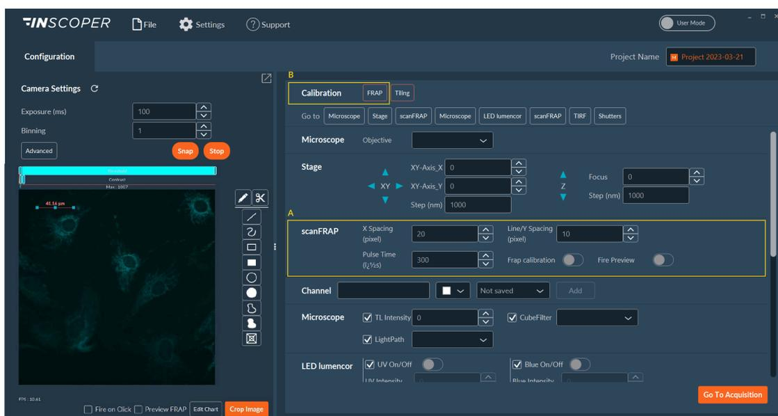
The **scanFRAP** section (A) in the **Configuration tab** allows you to adjust the point density (space between points) for photomanipulation. The X and Y spacing refers to the density of filled forms. For lines or unfilled forms, the line/Y spacing is considered.
