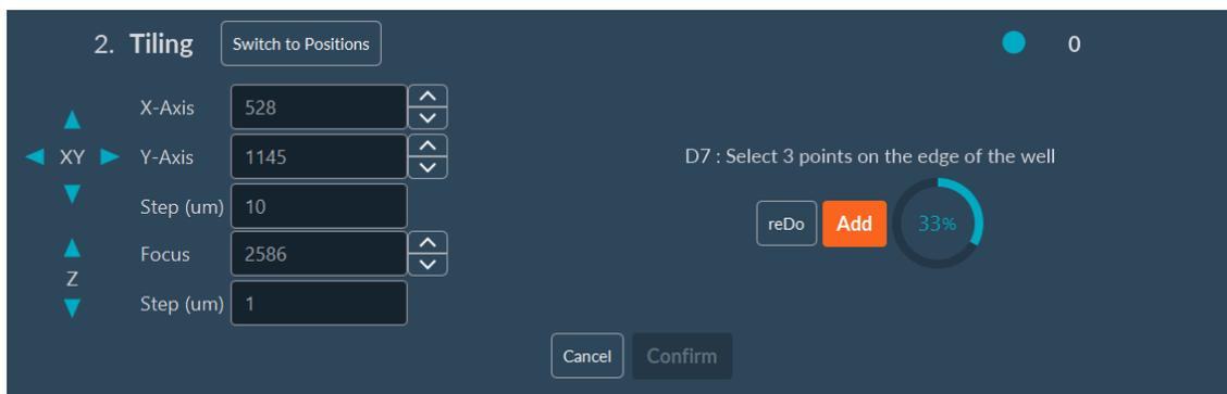
This step is needed to get precise positions of the well, and then to optimize the XY stage movements. To use the well plate feature:
