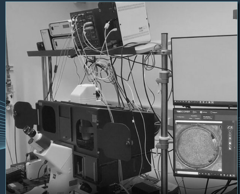
Ultra high-speed live cell image acquisition system (continuous motion imaging), Gaithersburg, Maryland, USA
